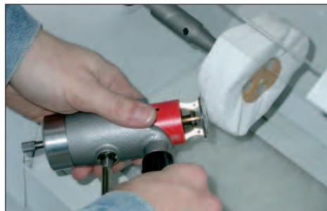
In case of voluntary blocking, just hold the base of the red vice.
